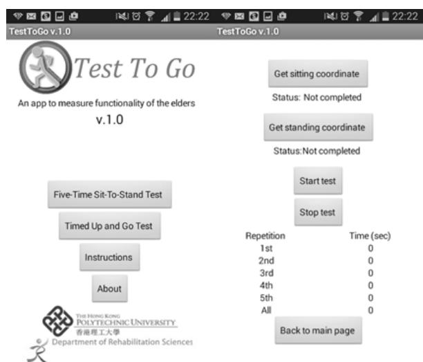
**Figure 1** Home page of the Test To Go mobile application that includes the FTSSTapp.
